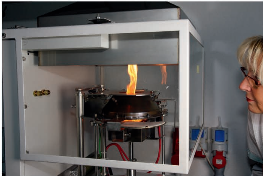
Cone-Kalorimeter-Messung/ Cone-calorimetry measurement
